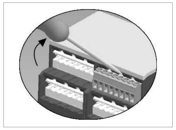
Do not remove the terminals by pulling the cables!
