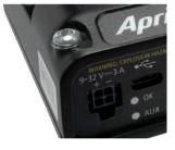
**Warning:** If the Aprisa LTE is operated in an environment where the ambient temperature exceeds 50°C, the Aprisa LTE must be installed within a restricted access location to prevent human contact with the enclosure heatsink.
