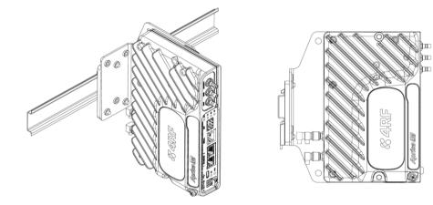
The Aprisa LTE has an earth connection point on the top left of the enclosure. Use the supplied M4 screw to earth the enclosure to a protection earth.
