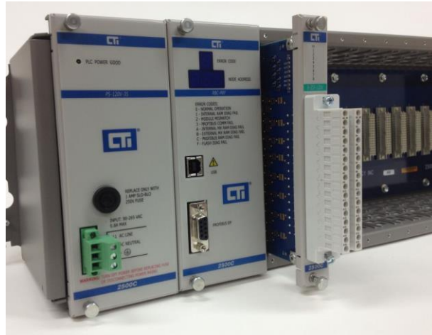
Figure 18 2500C-8-RTD Module Physical Installation Picture
