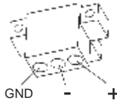
Figure 2.1: Terminal Block Pin Assignment
