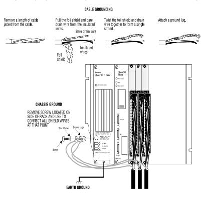
Figure 2.7 Shield Wire Termination
