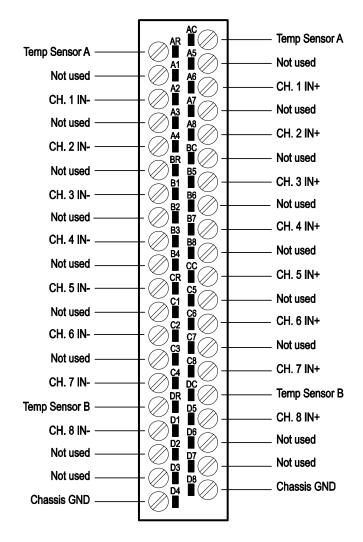
**Figure 2.3 Screw Terminal Connector Wiring**
