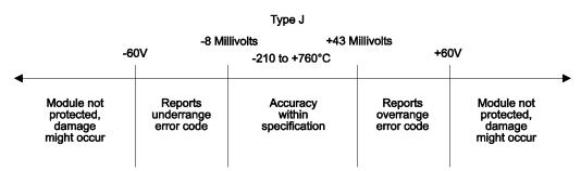
Figure 1.4 Effect of Voltage Input on Type J Thermocouple
