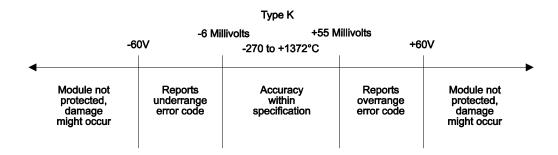
Figure 1.5 Effect of Voltage Input on Type K Thermocouple
