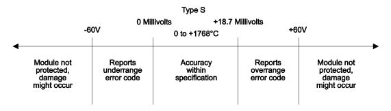
Figure 1.9 Effect of Voltage Input on Type S Thermocouple
