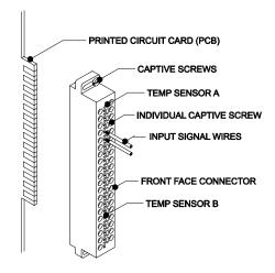
Figure 2.8 Input Connector Assembly
