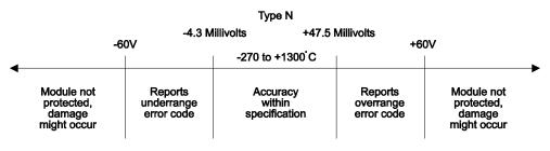
Figure 1.10 Effect of Voltage Input on Type N Thermocouple
