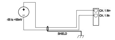
Figure 2.5 Millivolt wiring application
