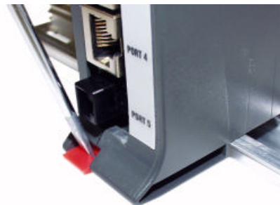
Figure 4. Removing the 3570 from the DIN rail
