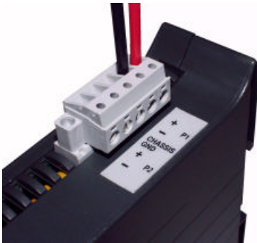
Figure 5. Single Power Supply Wiring
