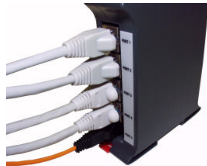
Figure 7. RJ45 and MTRJ cables on 3570-1F
