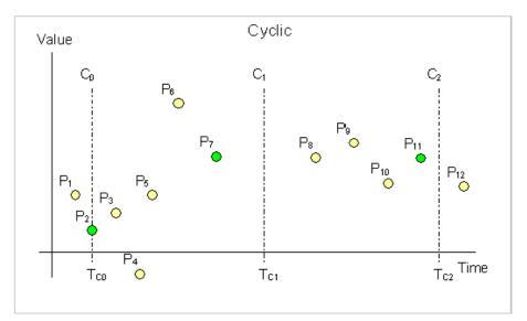
Data is retrieved over a period starting at  $T_{C0}$  and an ending at  $T_{C2}$ . Each dot in the graph represents an actual data point stored in the Historian. The Historian can return data from three cyclic intervals at  $T_{C0}$ ,  $T_{C1}$ , and  $T_{C2}$ .
