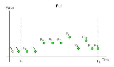
Data is retrieved in full mode with a start time of  $T_1$  and an end time of  $T_2$ . Each dot in the graphic represents an actual data point stored on the historian. From these points, the following are returned:
