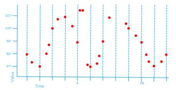
• **Cyclic storage** - Only values that occur at a specified time interval are stored. Using the same collected values as shown above, cyclic storage retains only the values represented by red dots.
