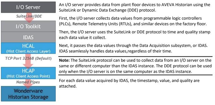
Then the values are sent through the Historian Client Access Layer (HCAL) to a Historian Client Access Point (HCAP) on the Historian server, and then to storage. HCAL is a client-side software layer that provides programmatic access to storage, retrieval, and system configuration functionality in the AVEVA Historian.
