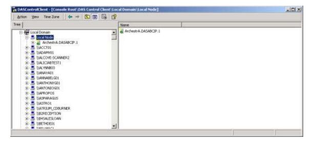
2. Highlight and expand the **XXX.DASABCIP.1** icon's tree view. It is located under the **Local Node** in the DAS Control Client Tree pane.
