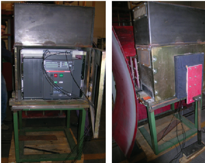
ABB Emax testing enclosures (ref. ANSI requirements)
