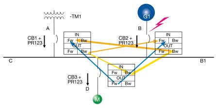
In case of fault in C, CB1 and CB2 are passed through by a current flowing in the same direction as the one set, whereas CB3 is passed through by a current with the opposite direction. No circuit breaker is blocked and consequently all the circuit breakers affected by the fault will trip according to the time settings of the protection S or I.
