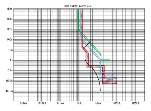
Here above, the set time-current curves for generator GS2 (black line), generator protection CB2 (red), motor protection CB7 (blue) and bus tie CB8 (green) are indicated.
