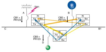
In the case of a fault in B, the circuit breaker CB2 is passed through by a current from busbar B1. This current flows in a direction against the one set. The DBout of CB2 "blocks" the DFin of CB1 and the DBin of CB3. In fact, current flows through CB1 in the same direction as the setting, whereas CB3 is passed through by a current opposite from the setting.
