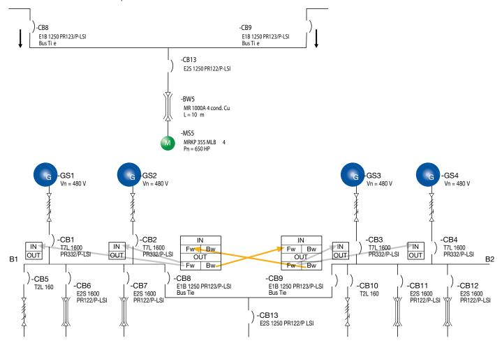
In the event of a fault on the busbar B2 the bus tie of busbar B1 must remain closed, while bus tie B2 must trip so that the fault is isolated.
