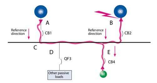
In this second case (fault on the supply side of CB2), only CB2 must trip:
