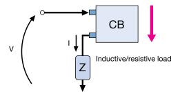
Once the power flow reference direction has been chosen, the flow of the positive reactive power towards the load (refer to the picture above) is the defined "forward" direction. On the contrary, the flow of the negative reactive power towards the load is the defined "backward direction". In this manner, because of the bond between reactive power and current, the forward and the backward directions are also defined for the current.
