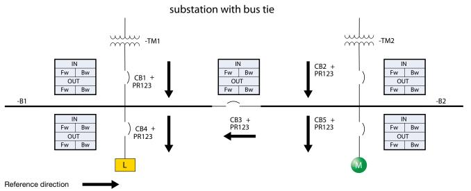
The presence of two or more MV/LV transformers and a bus tie closed on the LV busbars in a transformer substation allows the network to be managed with the transformers in parallel. This kind of configuration has the main advantage of allowing power supply even in the case of outage of one transformer. Thanks to SdZ D it is possible to keep half the busbar supplied with voltage even in the case of a fault on the other half of the busbar.
