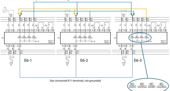
The terminals that must be connected are physically present (and clearly identified) in EMAX terminal box.
