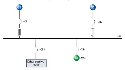
Consider an electrical scheme like the one above. The contribution of the motor to the maximum short circuit current is about 5 kA. The contribution to the short circuit by each generator is about 10 kA.
