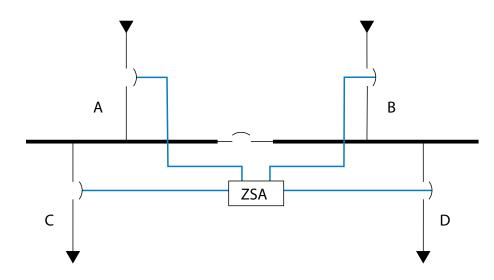
In fact, ZSA is a diode matrix that allows distributing the input blocking signal to the correct output without undesired signal returns. Look at the example below:
