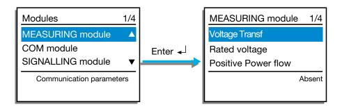
Choosing the power flow direction is simple. Entering in the measuring module menu (you can find it in the settings menu) and selecting "positive power flow" is possible to make a choice between
