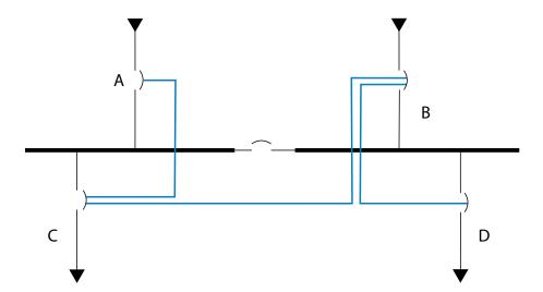
In fact, the lock signal coming from D would also be transmitted to A by means of the electrical continuity which is created between the different B-C and C-A interlocking connections.
