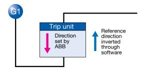
There is a default power flow reference direction on the circuit breaker, indicated by a red arrow. If it is necessary, it is possible to invert the reference direction through the software of the trip unit. Working in this way all the values measured with the PR123 and PR333 trip units will be assessed as they actually flow in the installation.
