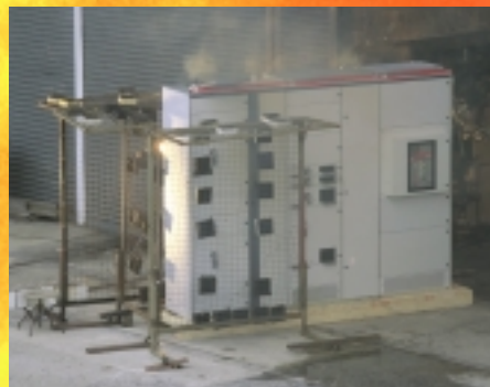
Low voltage switchgear during test (CRL97 665-11)
