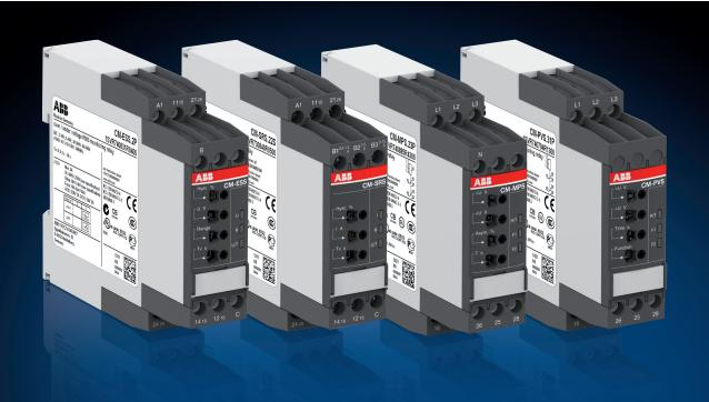
Measuring and monitoring relays Single- and three-phase
