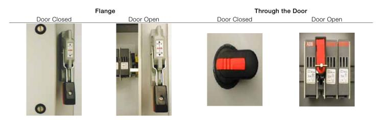
NFPA79 - 5.3.4.2 (1) Operating handle accessible with door in the open or closed position. UL508A - 66.6.3. (a) Readily accessible when the enclosure doors are in the open or closed position; UL508A - 66.6.3 (b) Installed so that its operation is not restricted by the enclosure door while in the open position;
