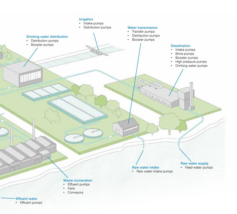
Regardless of the application, pumping water can be a demanding business involving problems such as water hammering when stopping the pumps, voltage fluctuations in the network when starting, and problems with jammed or clogged pumps. All of these problems need to be solved in order to keep the water facilities operational and in order to secure a reliable water management.
