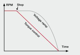
Comparing torque control with a normal voltage ramp
