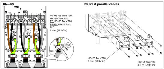
4. Frames R1...R3 and R6...R9: Install the control cable grounding shelf.
