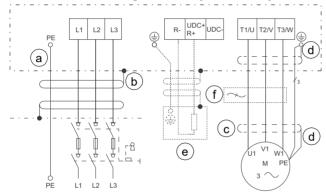
Note: NEC installation can include separate insulated conductors inside a conduit, shielded VFD cable in conduit, or shielded VFD cable without conduit. The normal dashed symbol (c) in this diagram represents the shield of shielded VFD cable. The same solid symbol (b) represents conduit
