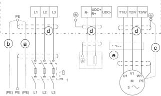
a. Two protective earth (ground) conductors. Drive safety standard IEC/ EN 61800-5-1 requires two PE conductors, if the cross-sectional area of the PE conductor is less than 10 mm<sup>2</sup> Cu or 16 mm<sup>2</sup> Al. For example, you can use the cable shield in addition to the fourth conductor.
