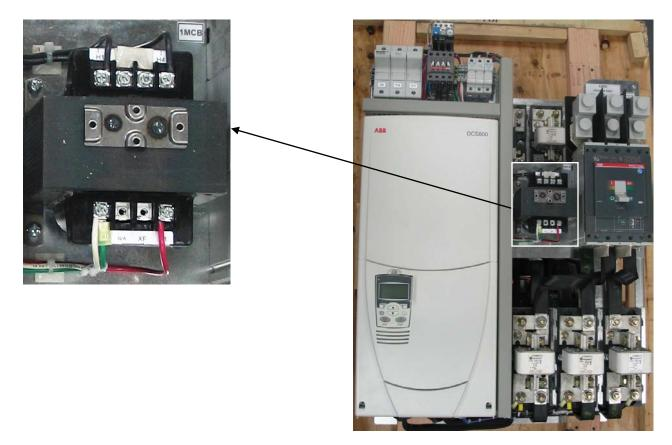
On the C frame drives built before May, 2013, the control transformer is located to the right of the drive module and is accessible without removing any other equipment.
