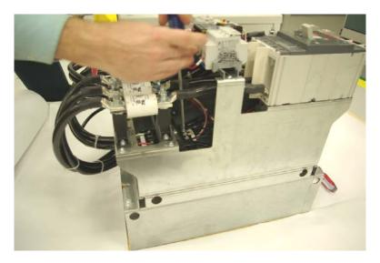
The control circuit transformer is located behind the main ac input fuses (F1,F2,F3). Access to the jumpers is above the main fuse mounting plate.
