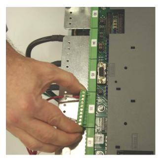
4. Remove the (4) drive module mounting screws and carefully move the module to allow access to the control circuit transformer. Avoid unnecessary stress on any power or control wires.
