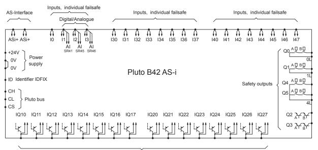
Failsafe inputs / Outputs (not failsafe) / Dynamic outputs
