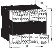
The connection block is removable without having to disconnect any cables. The units are assembled with a gap of at least 5 mm.
