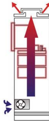
Airflow through cabinet via fans (negative/positive pressure)
