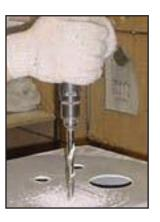
Using a drill with a positive rake angle and thin points or split points can help reduce cutting pressure. Feed rates must also be constant and may even be reduced upon exiting from a hole to reduce flexing of the part when the drill exits. Using a solid back surface to support the part when drilling can also aid in reducing delamination and chipping. Caution on polycarbonate to not generate enough heat that the material starts to melt or string.
