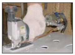
saw or fine toothed saw will provide the highest quality cutout with minimal edge chipping.
