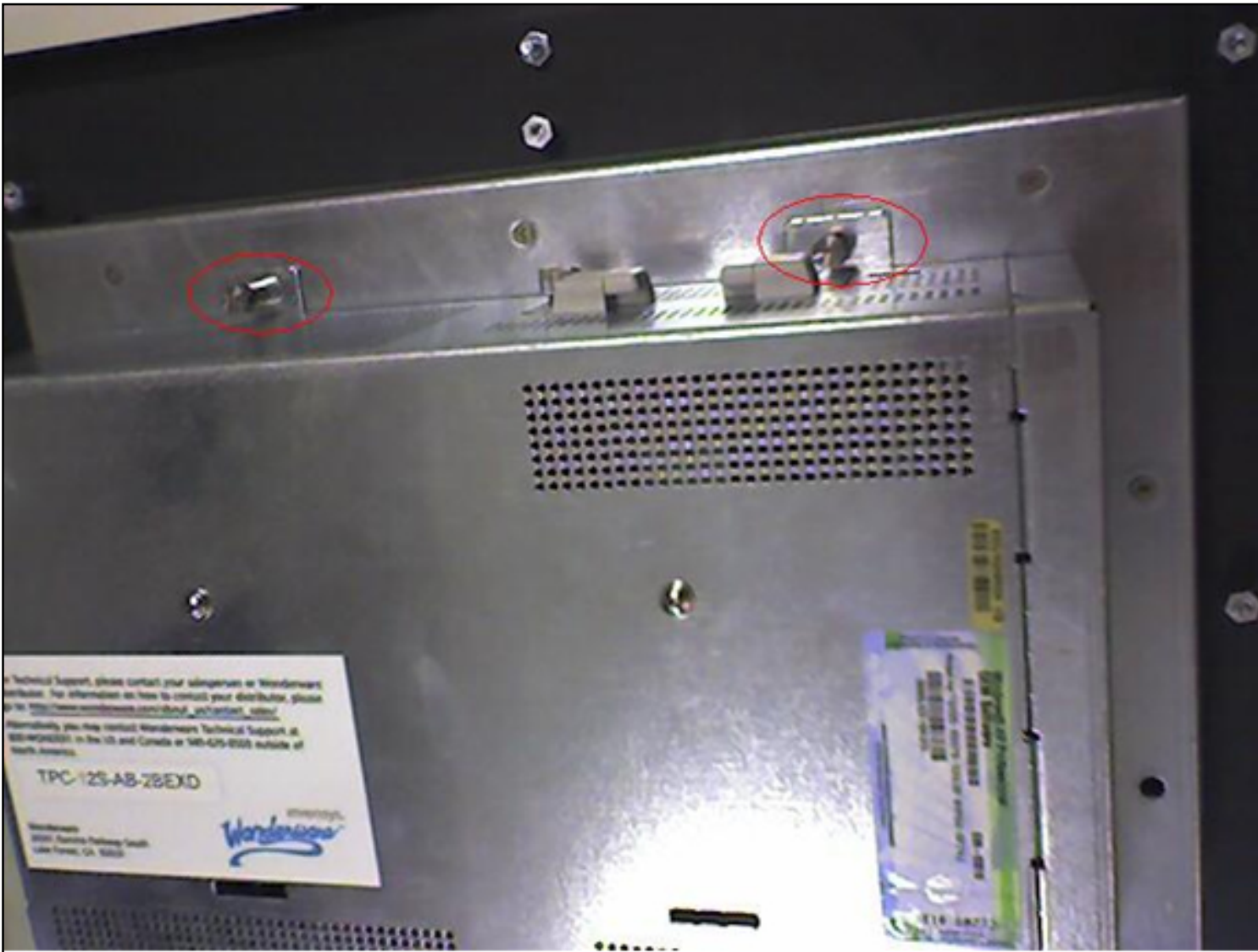
Figure 1: Unscrew and Remove the Bezel
