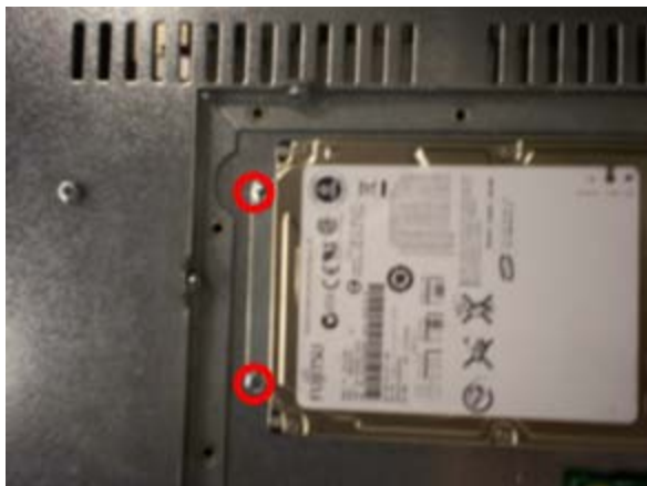
FIGURE 3: REMOVE THE MOUNTING PLATE SCREWS
