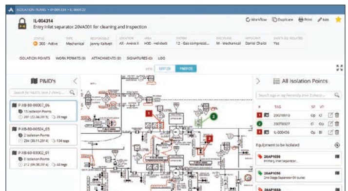
Create isolation plans by direct visual interaction with intelligent P&IDs
