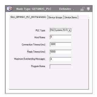
You can create a maximum of 128 GEFANUC\_PLC objects from the **New\_GESRTP\_PORT** branch. This maximum number can be of a single type of PLC or a combination of several types of PLCs.
