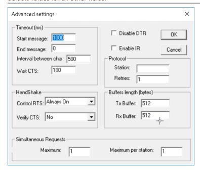
The following parameters are configurable in the TI500 Communication Driver:
