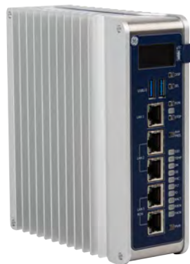
Figure 6. GE Outcome Optimizing Controller (RX3i CPE400)
