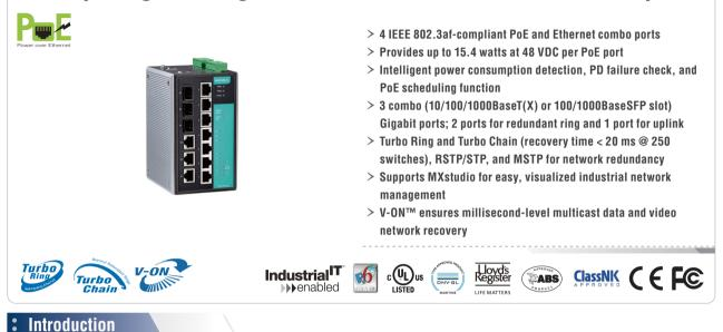
The EDS-P510 Series Gigabit managed redundant Ethernet switches have 4 10/100BaseT(X) 802.3af (PoE) compliant Ethernet ports and 3 combo Gigabit Ethernet ports. The EDS-P510 switches provide up to 15.4 watts of power per PoE port, and allow power to be supplied to connected devices (such as surveillance cameras, wireless access points, and IP phones) when AC power is not readily available or is cost-prohibitive to provide locally. The EDS-P510 switches are highly
