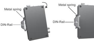
To remove the ICF-1170I series from the DIN-rail, simply reverse Steps 1 and 2 above.
