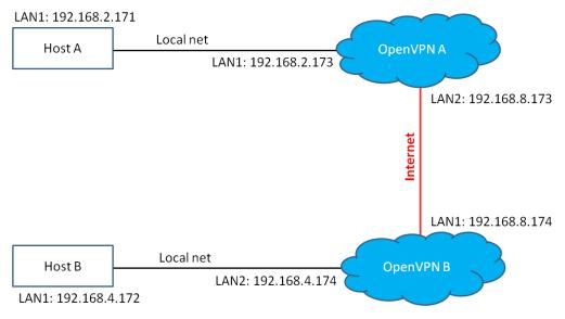
Host A (B) represents one of the machines that belongs to OpenVPN A (B). The two remote subnets are configured for a different range of IP addresses. When this setup is moved to a public network, the external interfaces of the OpenVPN machines should be configured for static IPs, or connected to another device (such as a firewall or DSL box) first.
