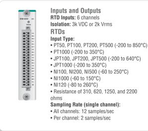
Resolution: 0.1°C or 0.1 ohms Accuracy: ±0.1% FSR @ 25°C ±0.3% FSR @ -40 and 75°C Input Impedance: 625 kilo-ohms (min.) Wiring: I/O cable, 16 AWG (max.) Connector: Spring-type terminal block Environmental Limits Operating Temperature: -40 to 75°C (-40 to 176°F) Power Requirements Input Current: 201.5 mA @ 3.3 VDC MTBF (mean time between failures) Time: 571,446 hrs Standard: Telcordia SR332
