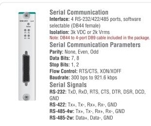
Physical Characteristics Connector: DB44 female Environmental Limits Operating Temperature: -40 to 75°C (-40 to 176°F) Power Requirements Input Current: 375.8 mA @ 3.3 VDC MTBF (mean time between failures) Time: 596,611 hrs Standard: Telcordia SR332
