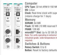
Computer CPU Type: 32-bit ARM 9 192 MHz CPU **OS:** Linux **Clock:** Real-time clock with super capacitor (retains charge for 7 days) Memory SDRAM: 64 MB Flash: 32 MB (10 MB reserved for user) FRAM: 128 KB microSD<sup>™</sup> Slot: Up to 32 GB (SDHC compatible) Note: For units operating in extreme temperatures, industrial-grade, wide-temperature microSD cards are required. **Switches & Buttons** Rotary Switch: 0 to 9
