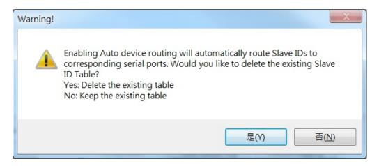
Click **Yes** to delete the existing (factory default or user-set) routing table; the auto routing mechanism will automatically find the correct serial port that connects the target Modbus device. Moreover, if a device is added to the gateway later, the gateway can also route it correctly. Note that the routing table will be clear as illustrated below.
