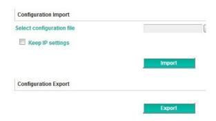
Once the file has been saved, it can be imported into your target unit to duplicate the same settings. Select the target unit first and then click the **Import** button to complete the import action.
