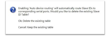
Click **OK** to delete the existing (factory default or user-set) routing table; the auto routing mechanism will automatically find the correct serial port that connects to the target Modbus device. Moreover, if a device is added to the gateway later, the gateway can also route it correctly. Note that the routing table will be clear as illustrated below.
