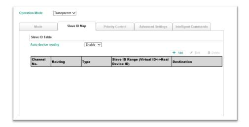
Once the Modbus Master starts to send Modbus requests, the gateway will auto-detect the routing and show results in the web console.
