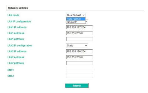
**Dual Subnet** mode allows the gateway to have two different IP addresses, each with distinct netmask and gateway settings. **Single IP** mode allows users to use the same IP address on both Ethernet ports.
