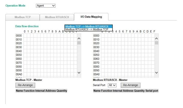
In agent mode, you need to manually set Modbus commands one-by-one and assign a gateway memory address for storing this data. We recommend using **I/O Data Mapping** to check the memory address of each command.
