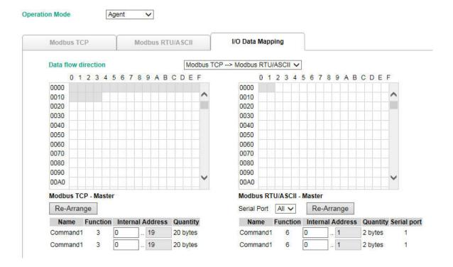
You can click on the **Re-Arrange** button to automatically address the internal address. The update internal address will become as follows:
