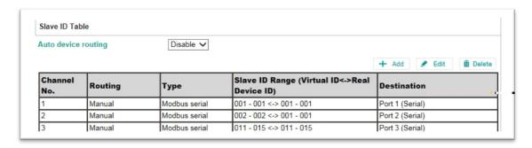
Now, the Modbus master can send a request with slave ID 1 to the Modbus device A connected to serial port 1 as well as sent a request with slave ID 2 to the Modbus device B connected in serial port 2.
