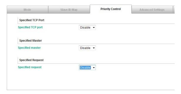
Priority control is designed for requests that are sent to Modbus RTU/ASCII slaves. Since Modbus RTU/ASCII slaves cannot handle multiple requests, the Modbus gateway must send each request individually and wait for the response before sending the next request. As requests stack up, the response time can suffer. This can cause problems for certain critical requests that require an immediate response.
