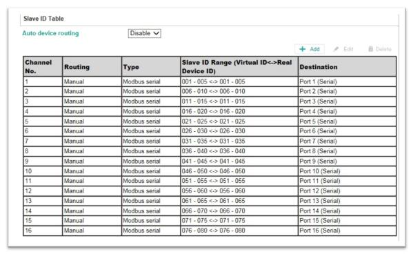
Select the first channel and click **Edit**. The *Slave ID* here represents the Virtual ID recognized by the Modbus master.
