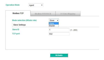
Modify the Slave ID settings to match the system requirements. The default TCP port for Modbus TCP is 502, so you may need to modify if there is a firewall in place.
