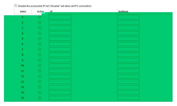
These settings are used to restrict access to the module by IP address. Only IP addresses on the list will be allowed access to the device. You may add a specific address or range of addresses by using a combination of IP address and netmask, as follows:
