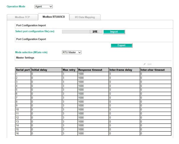
The MGate MB3660 also provides several advanced settings for specific application requirements. The following settings are optional for most applications. It is suggested to use the default settings to test the MGate MB3660.
