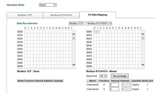
To rectify the error, click **Command4** to change its starting address from 2 to 3.
