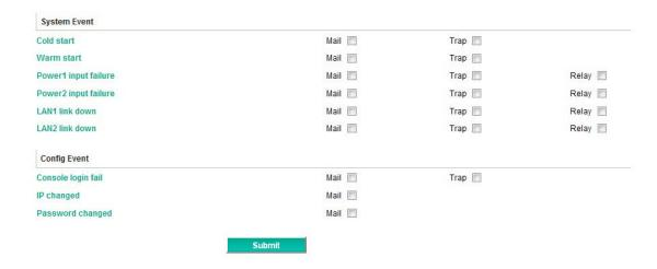
Auto Warning is triggered by different events. When a checked trigger condition occurs, the MGate can send e-mail alters, SNMP Trap messages, or open/close the circuit of the relay output and trigger the Fault LED to start blinking. To enable an e-mail alert, configure the e-mail address on the E-mail Alert page. Likewise, to enable SNMP Trap alerts, configure SNMP trap server on the SNMP Trap page.
