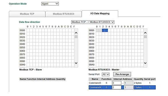
Once the change has been made, each of the two commands will be allocated to unique address ranges in the gateway's memory. That is, the address for command 3 will be in the range 0 to 1, whereas command 4 will be in the range 2 to 3.
