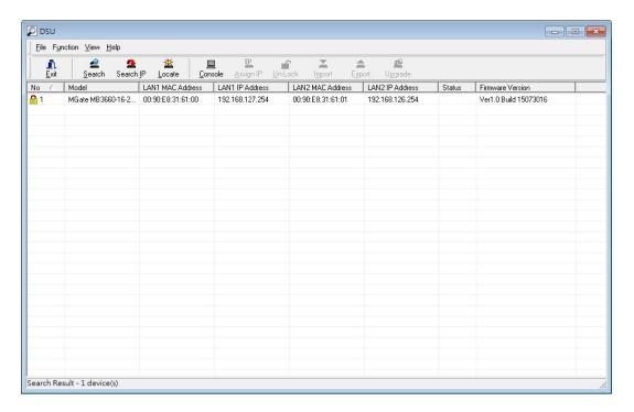
When the search is complete, every MGate MB3660 found on the LAN will appear in the DSU window. The MAC address, IP address, and Firmware version of each unit will be shown. Select the one you would like to configure.
