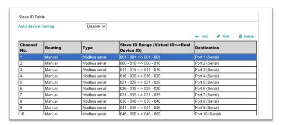
Then, select the second channel and click **Edit**. Since the virtual ID recognized by the Modbus master side is 2, and the real slave ID of the device B is ID 1, the offset should be set as -1.
