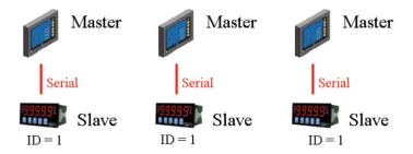
The MGate MB3660 can connect to each serial slave so Ethernet SCADA masters will be able to control them. However, since slave IDs cannot be repeated in a system, we will need to change the IDs of some of the slaves in order to integrate them into a single network, as follows:
