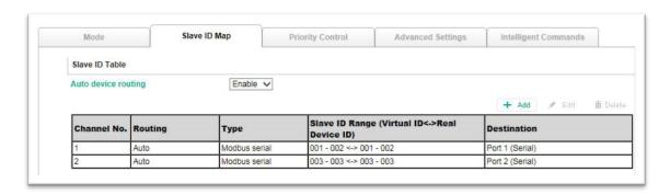
This snapshot shows the routing mechanism is in *Auto* mode, and the gateway detects that slave ID 1 and 2 are connected to port 1 and slave ID 3 is connected to port2.
