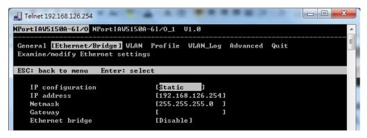
8. Press ESC to return to the menu. When prompted, press Y to save the configuration changes.
