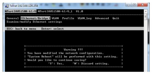
The NPort will reboot with the new IP settings. You can telnet to the new IP to log in again.
