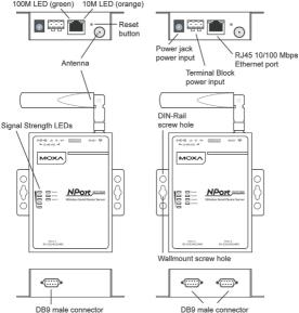
**Reset Button**: The reset button is used to load the factory default settings. Use a pointed object to hold the reset button down for five seconds to load the factory defaults.
