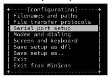
4. Select **A** to change the serial device. Note that you need to know which device node is connected to the RISC computer.
