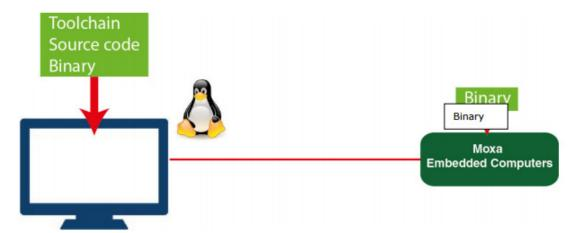
To ensure that an application will be able to run correctly when installed on Moxa computers, you must compile the application and link it to the same libraries that will be present on Moxa computers. This is particularly true when the RISC Cortex processor architecture differs from the CISC x86 processor architecture of the host system, but it is also true if the processor architecture is the same.
