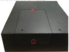
2. Remove the cover to access the SD-card slot and the mSATA socket.  $\label{eq:msata} \text{mSATA}$
