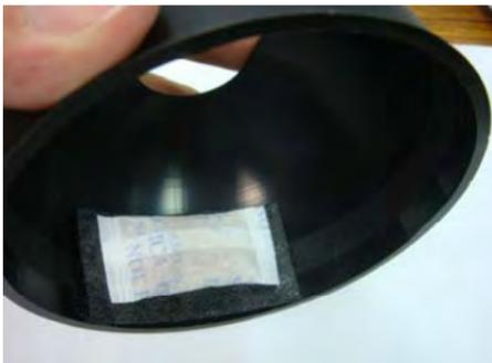
**NOTE** The effect of the silica gel desiccant will decrease after being used for particular time period. Silica gel desiccants are commonly available, and can be replaced with the hook fastener.
