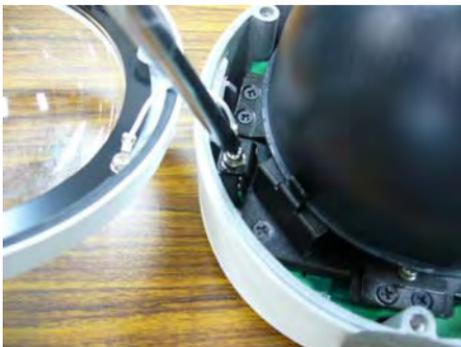
**Step 2: Remove the inner case.**
