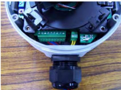
**NOTE** Be sure to arrange the cables carefully to make sure that all cables are connected properly. We recommend connecting the Ethernet cable first, and then the 9-pin terminal block. Connect the 2-pin terminal block last.
