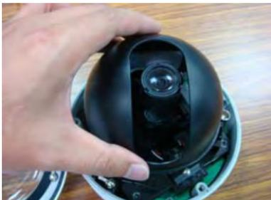
**Step 3: Remove the IP camera module.**
