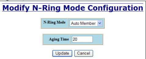
The N-Ring Aging Time has a default of 20 seconds and is separate from the Bridging Aging Time. N-Ring Aging Time is used when the switch is an N-Ring Manager, N-Ring Multi-Member, or becomes an active N-Ring Member, and in any case N-Ring status includes for example:
