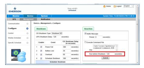
**3.** We have built the **command.KVM** script file to shut down the guest OSes, so you have to change the file name from command.ESX to command.KVM in the **Execute Command** File. Please then check the **Execute Command File** checkbox to enable shutdown the guest OSes.
