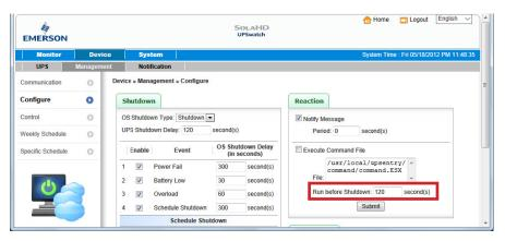
**3.** We have built the **command.Xen** script file to shutdown the guest OSes, so you have to change the file name from command.ESX to command.Xen in the Execute Command File. Please then check the **Execute Command File** checkbox to enable shutdown the guest OSes.
