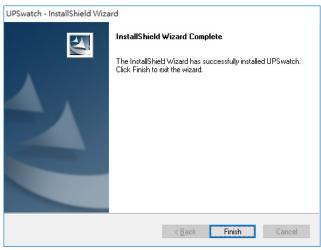
7. Once the installation is complete, UPSwatch will automatically start the service program and add an icon to the task bar. A dialog box will pop up to ask if you want to configure the basic parameters via console. If you are not operate a Windows server core operating system then you can ignore this. Just press "No" to finish the installation. Press "Yes" to launch the console configuration in the shell mode. See chapter 3 for more details.
