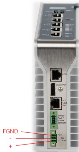
Figure 8: 24 VDC Power Input Connector
