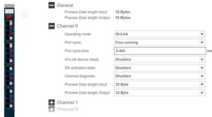
Figure 296 IO-Link master Parameterization
