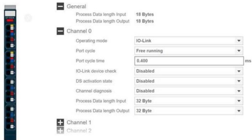
Figure 295 IO-Link master Parameterization
