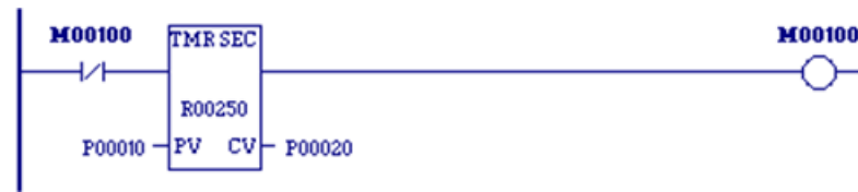
Figure 43: Ladder Logic for Synchronizing Timer
