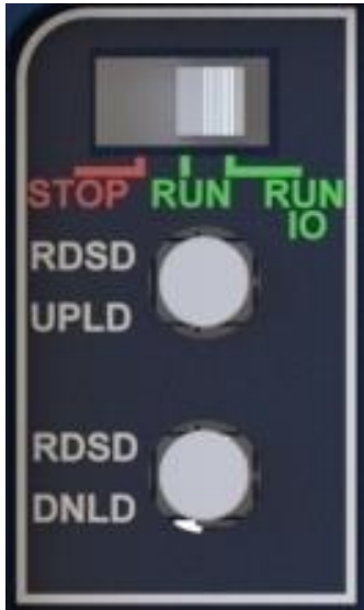
Figure 2: CPE330 RUN/STOP Switch and RDSD Switches
