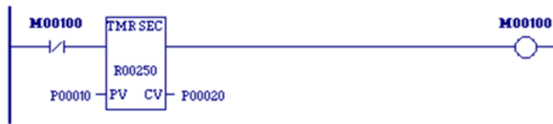
Figure 43: Ladder Logic for Synchronizing Timer
