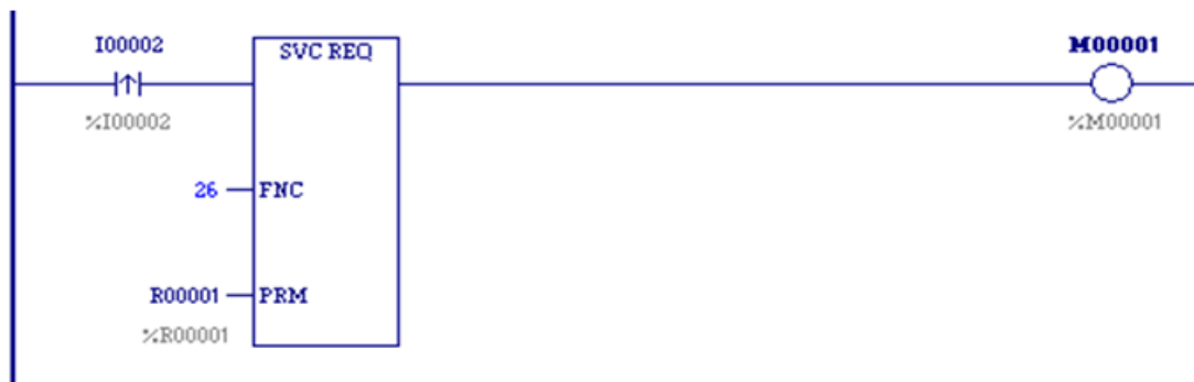
Figure 41: Ladder Logic for Role Switch (SVC_REQ 26)
