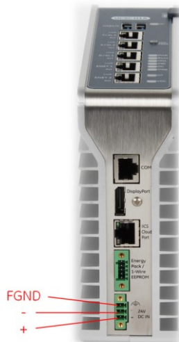
Figure 8: 24 VDC Power Input Connector
