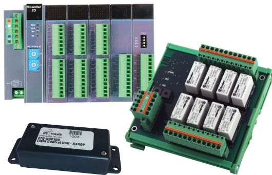
Wired Control and Monitoring CsHop networks repeat at each device for long reliable runs over standard cat5 cable. Ethernet and CAN based IO provide lighting control, temperature monitoring and more.
