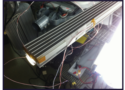
Initially with no dust, measurements were recorded after approximately 1 hour of run time and temperatures were stable. LEDs = 77.2°C, Phosphor = 51.5°C, Housing = 52.8°C
