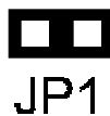
OIU327, OIU327-24, OIU357, OIU357-24 Jumper Setting to Provide +5V to the RS-422/485 Port
