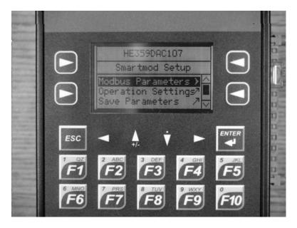
Note that the top line in this screen should accurately reflect the type of Smartmod connected, in this case a DAC107.
