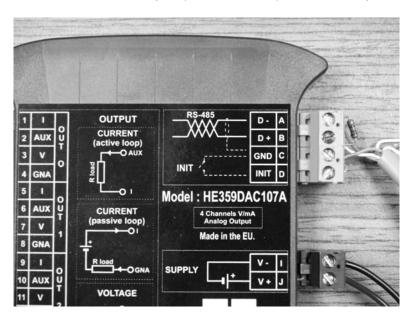
Place a jumper from INIT D to GND C...
