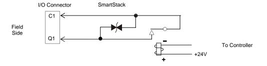
Specification for transient voltage suppressors (transorbs) used on output circuitry is 400 VDC, bidirectional 1500 W.
